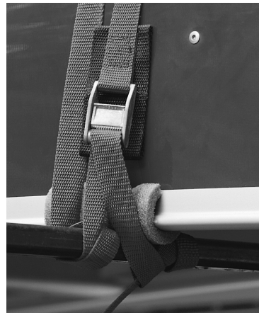
Cam-type straps hold the canoe more securely than ropes and are easier to use.
